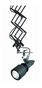
Given its fixing position, the asymmetric weight of the lamp attached to the pantograph would make it slant. Both hang vertically thanks to the balance point counterweight ROTAI between the pantograph and the lamp.
